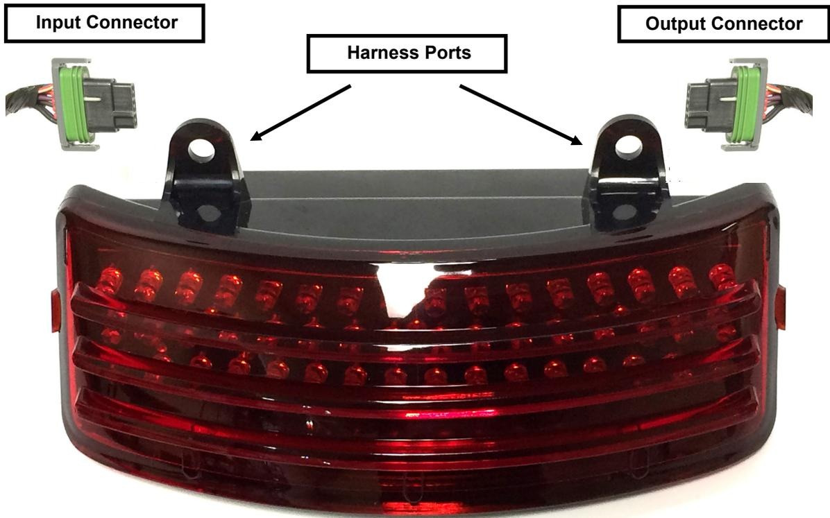
Plug the harness connectors into the new Tri-Bar, noting the rectangular ports on the back side of the unit. Left side should be going to the bike, the right side is the output to the turn signals. Make sure that the connector orientation is correct going into the ports, they are keyed one way, if the connector does not want to snap in, flip it around and try it again.
